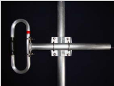
1/4 - wave spacing (1.90 - 2.25 dBd gain) (Offset pattern)
